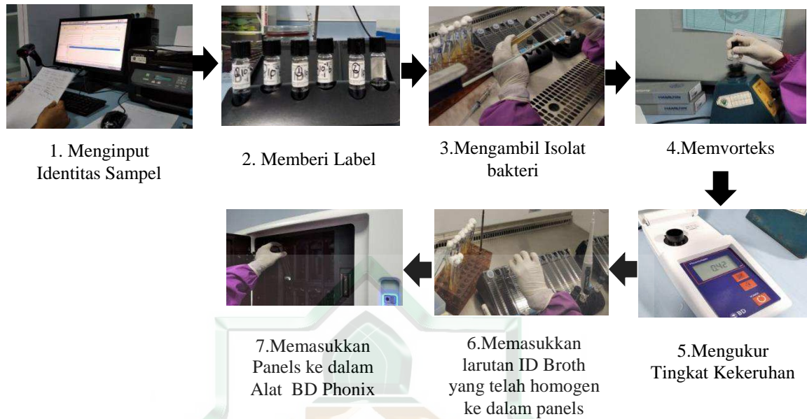
Gambar 3.1 Alur kerja microbiology analyzer .
